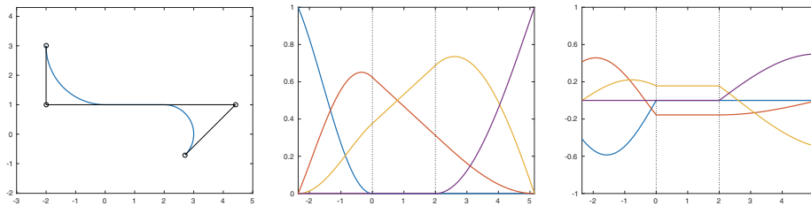
FIG. 8.2. A profile consisting of two circular arcs connected by a straight line defined in Example 8.2 (left column), together with the C^1 GTB-splines used in the representation (middle column) and their first derivatives (right column). Knot positions are visualized by vertical dotted lines.
